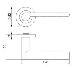
Lever on a concealed fix threaded rose. A straight flat bar lever with a smooth rounded end. Part of the Steelworx range in grade 304 Stainless Steel. Comes with a 10 year mechanical guarantee and is Fire door rated.
