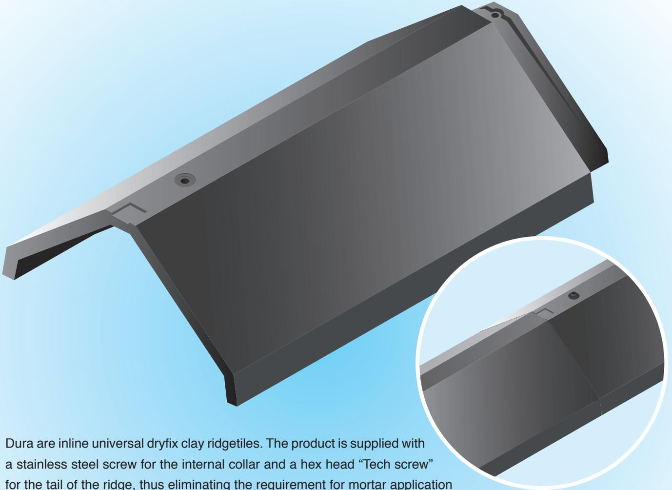
Dura are inline universal dryfix clay ridgetiles. The product is supplied with a stainless steel screw for the internal collar and a hex head “Tech screw” for the tail of the ridge, thus eliminating the requirement for mortar application and providing a very quick and robust fixing.
