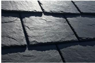
The Del Carmen Slate was formed 505 million years ago. A true geological slate exhibiting a range of properties that make it highly suitable for use as roofing slate. The quarry is situated about 3 miles west of the village of La Bana in the Cabrera Mountains, Spain approximately 4,750 feet above sea level.
