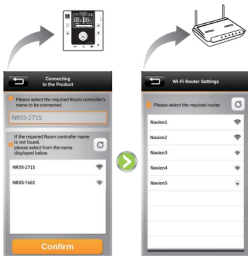
Connect your room controller to Wi-Fi connection thru your wireless router
