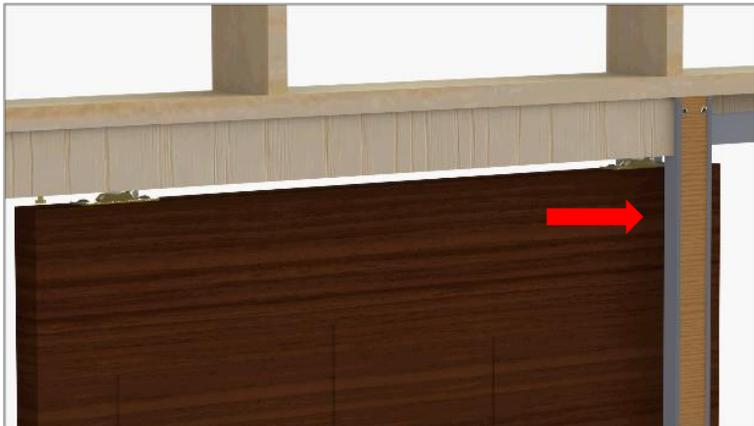
Slide the door inside the pocket to ease mounting the second door plate.
