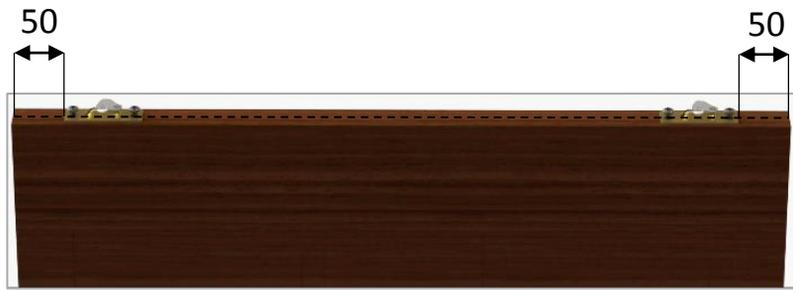
Attach the door plates on the top of the door at 50mm from the edges.
