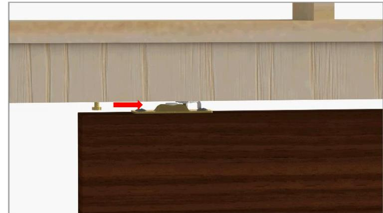
Insert hanger pin into the second door plate slot.
