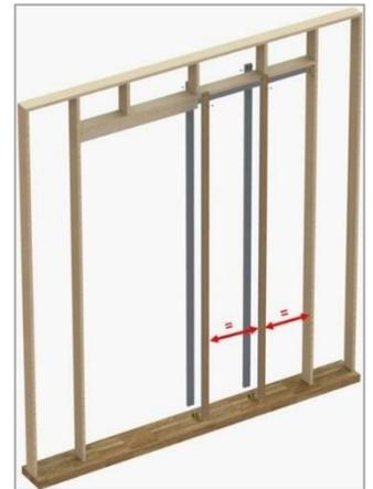
If kit supplied has 6 split studs, the first set of 2 will be placed on the track and butted up to the head.
