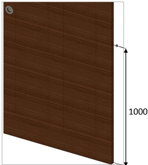
Attach bumper at the back of the door at 1000mm from the bottom.
