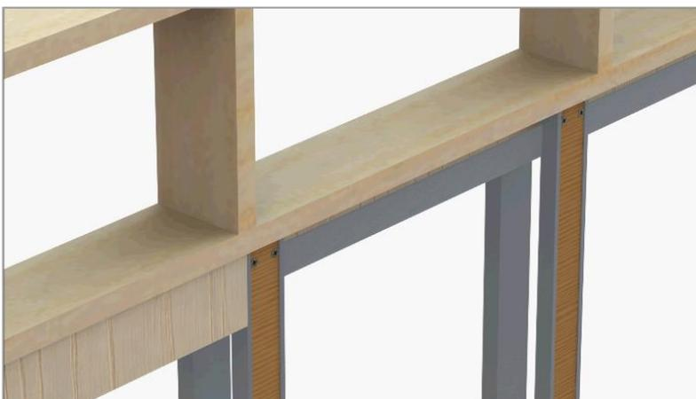
Fix the first set of split studs by butting them to the header and the track, make sure they are in a levelled position, and fix them with screws.
