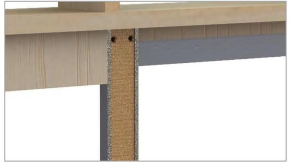
Place a split stud on the track and butt it up to the head, pre-drill and countersink holes for fixing screws, in the wood header NOT THE TRACK. Repeat the step for all the split studs.
