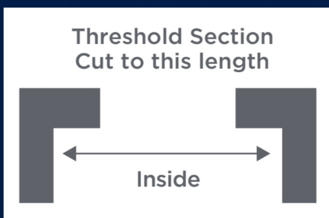
2. This sill requires an underdoor clearance of 30mm. If necessary, remove door and trim to allow for this.
