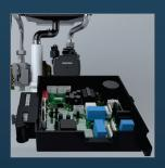
Coated PCB Water-Resistant circuit board. (IPX5D)
