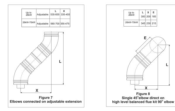
High Level Balanced Flue Kit
