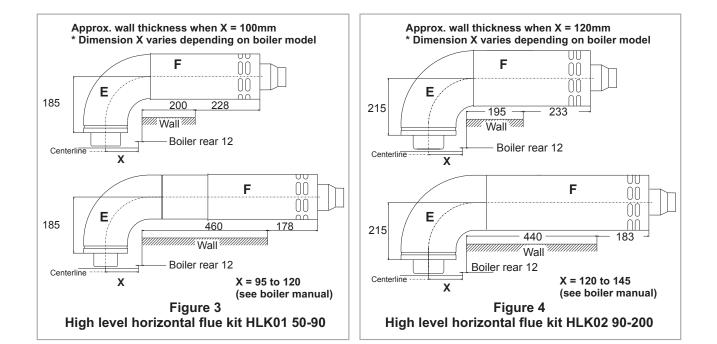
High Level Balanced Flue Kit
