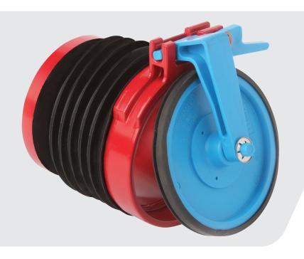
To prevent foul water flowing back from the blocked sewerage system to flood the property from the inside via toilets, plug holes and waste pipes. These unique and patented Retrofit Non-Return Valves can be simply pushed in to the existing pipework, whether plastic or clay, at the property's inspection chamber. The valves can be fitted in minutes and do not require any specialist expertise or equipment.
