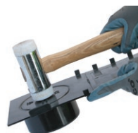
Removing knockout panel
