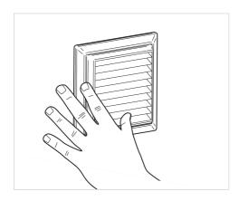
**3.** Clip the outer grille/cowl/gravity flaps into the wall-plate. If fitted, ensure that the gravity flaps move freely
