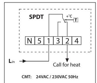
Wiring diagrams above are shown for heating applications.
