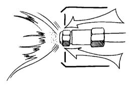
Oil sprayed from a nozzle placed too far back will be caught by the combustion head and may result in oil flooding from the burner tube. Here, it must be pointed out that the higher the fan pressure the plant works with the more accurate must the oil nozzle be located in relation to the burner tube, ignition electrode and combustion head. These remarks principally concern plants which run at 2800 rev/min.
