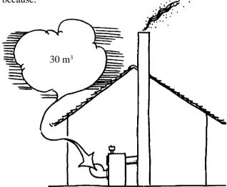
There is a lack of ventilation in the boiler room, i.e. sufficient air is unable to enter the boiler room and the burner fan cannot "breathe". A normal domestic oil-heating plant MUST receive approximately 30 m³ air per hour. If the fan is prevented from receiving this amount of air, combustion will rise to soot formation.
