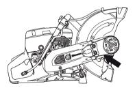
Rotate the bearing housing to opposite direction and reassemble the stop.
