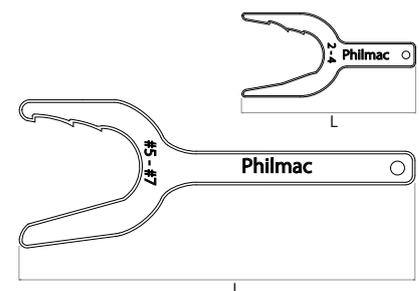
3G fittings can be installed using standard plumbing tools including Multi-grips or a Wrench. Some customers prefer to use a dedicated spanner and Philmac offers two designs. The classic C spanner and the new Y spanner are both available.
