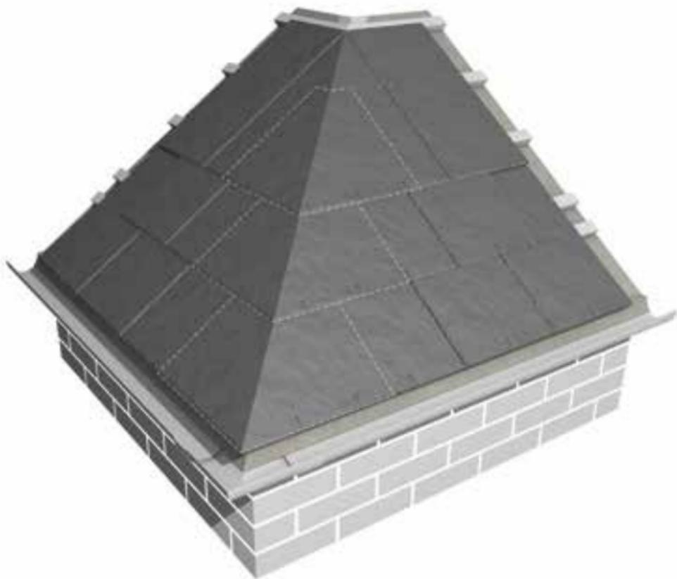
Close mitred hip constructions should not be used on roof pitches below 35°.
