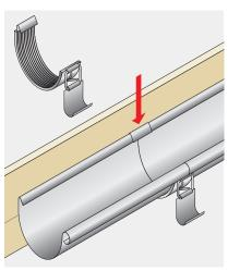
An EDPM rubber sealed union connector is used to connect the gutter lengths and angles together. Locate the union connector over the rear edge of the gutter.
