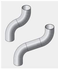
Offsets are achieved using 2/no 70° bends, with larger offsets being made by inserting a pipe length between the two bends.
