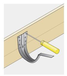
Generally position the fascia brackets at 915mm centres, using at least 3 brackets per gutter length. Use 2 screws on both the left and right fixing options and 1/no underneath the gutter securing tab.
