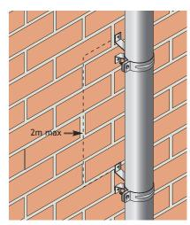
6. Downpipes should be installed using at least 2/no pipe clips per length. Mark out the clips locations and level with a sprit level or plumb line. Open the tightening screw to allow the pipe to be inserted, close the clip and re-tighten, making sure not to over tighten and damage the downpipe.
