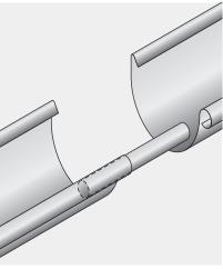
3. A bead connector is used to join two lengths of gutter. Insert the connector into the front roll of each gutter length. Allow for a 4mm expansion gap.
