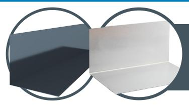
Aluminium soakers are for use when forming a pitched roof against an existing wall. Pre-fabricated to a 90 degree angle, soakers are inserted between successive courses to make a waterproof joint. A lightweight and durable alternative to lead.
