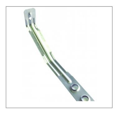
The BTS and SWT are wall ties used to restrain the external brickwork back to the building structures, while maintaining a clear cavity. The BTS and SWT offer an outstanding combination of performance and cost in a wall tie for use with timber frame or SIP (Structural Insulated Panels). Accommodates movement in timber frame and SIP structures allowing up to 24mm of movement.
