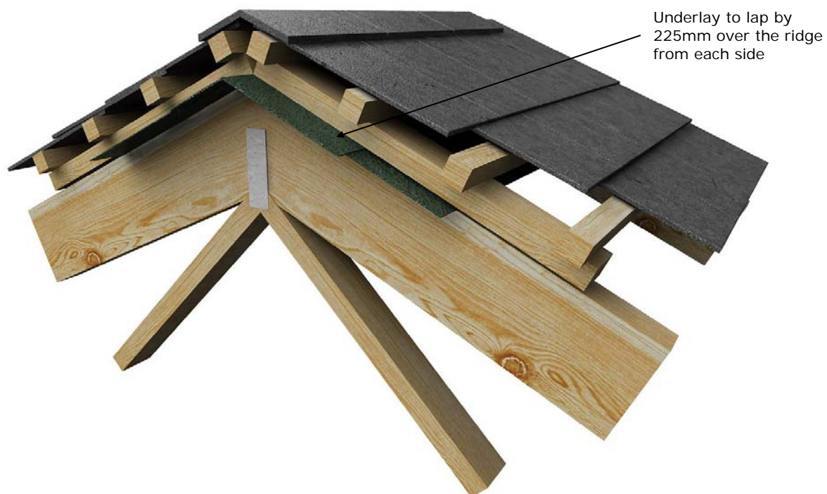
Figure 5: Sealed cold roof ridge detail
