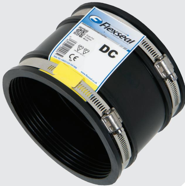
Flexseal Drain Couplings are used to connect, repair and maintain drainage systems and other small diameter non-pressure pipelines. Available to suit any pipe material up to 275mm outside diameter, Drain Couplings are designed for use in drainage systems where the resistance to earth loads (usually provided by a Standard Coupling) is not required.
