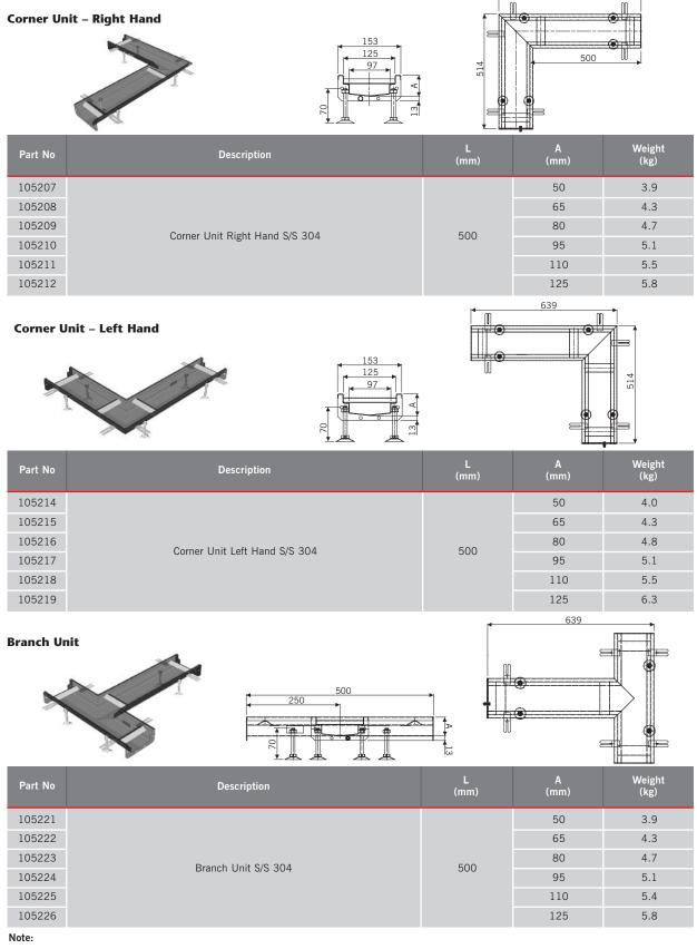
All channels are supplied complete with levelling feet, fixing ties, neoprene gaskets and fixings.
