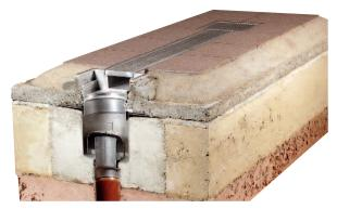
Prepare haunching on screed base working mix under channel and gully top flange. Lay levelling screed and lay tiles in cement bedding.
