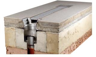
Fit the ACO Vinyl Seal® rigid extrusion and flexible seal system to channel and gully edge as described on pages 41-42. Prepare haunching.
