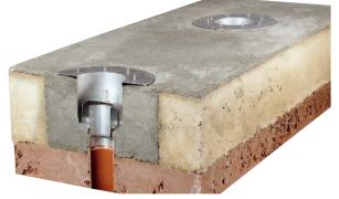
Backfill gullies with concrete and float to flange level.
