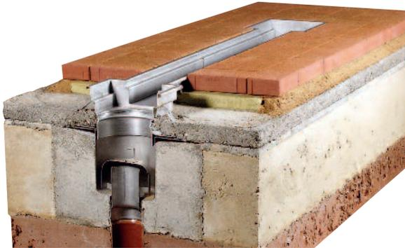
Prepare screed base working mix under channel and gully top flange and lay block paviors on 300mm wide epoxy surround to prevent movement. Set paviors 3mm maximum above channel edge. Complete paviors on compacted sharp sand bed.
