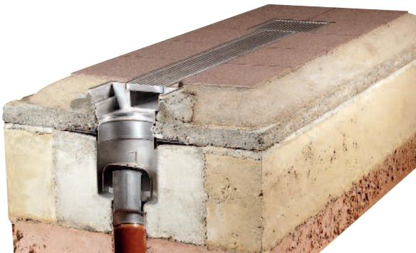
Prepare haunching on screed base working mix under channel and gully top flange. Lay levelling screed and lay tiles in cement bedding.
