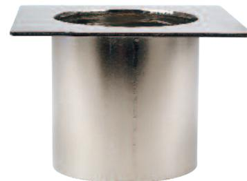
Electropolishing is ideal for producing a uniform, highly reflective lustre with an extremely smooth finish even on the most complex product contours. This is a well proven method of polishing and is achieved by an electro-chemical process which is essentially the reverse of electroplating.
