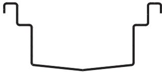
Suitable for tiled, concrete and epoxy resin floors in pedestrian and light industrial applications. Suitable for Load Class A15 & B125 to BS EN 1433.
