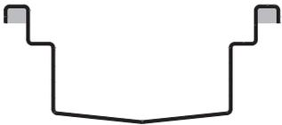
The underside of the channel can be infilled with a PVC strip to provide additional strength in dense traffic areas. PVC Infill is supplied loose for installation on site. Required for Load Class C250 to BS EN 1433.
