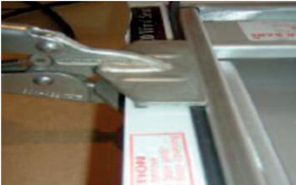
Using the Sheet Plier Grip Wrench, proceed along the channel edge inserting the black flexible seal.
