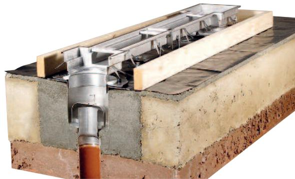
Taking into account finished floor materials and thickness (sharp sand, paviors, tiles, vinyl etc) construct shuttering for the levelling screed. Pour screed and remove shuttering.
