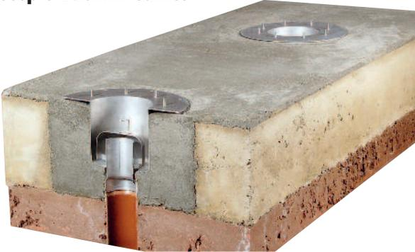
Backfill gullies with concrete and float to flange level.
