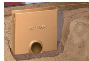
Access or sump unit must be fitted in order to allow subsequent access for maintenance and cleaning. If outletting from access unit knock out pre-formed outlet from the inside, fit PVC-U Ø110mm union, connect to outlet drainage pipework and position on C25 concrete bed. If installing sump unit follow above steps from fit PVC-U Ø110mm union.
