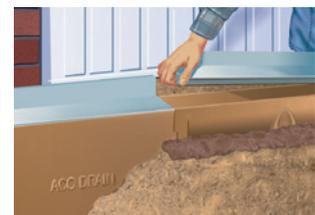
With Brickslot covers fitted haunch around channels with concrete. Bricks/paviours should be laid in Epoxy or Polymer Modified Mortar for lateral stability. Final surface to be 3-5mm above slot.
