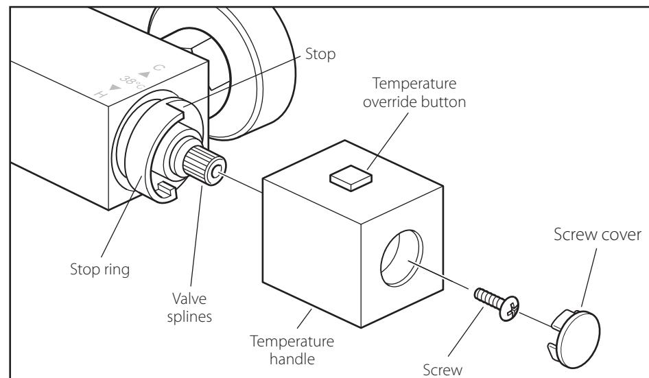
The valve has been factory set under balance pressures and hot water supply at 65° C. When your specific operating conditions are significantly different from the above, the temperature of the water may vary from the setting.
