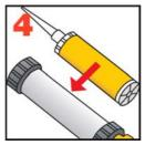
Place the cartridge into the gun and start application
