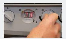
Turn the Central Heating control to set your temperature (this will display for a few seconds). This figure is how hot your
